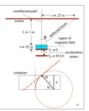
Using the conservation of energy through the accelerated portion of the flight:
